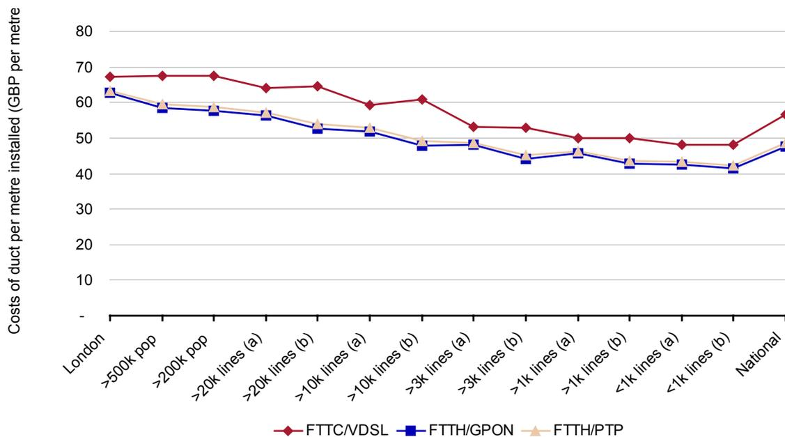
Figure A.8: Average costs of constructing new ducts [Source: Analysys Mason for BSG]
