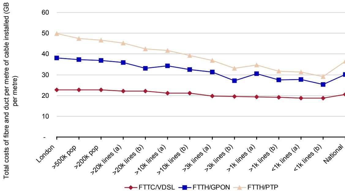
Figure A.9: Average cost per metre for fibre and ducts [Source: Analysys Mason for BSG]
