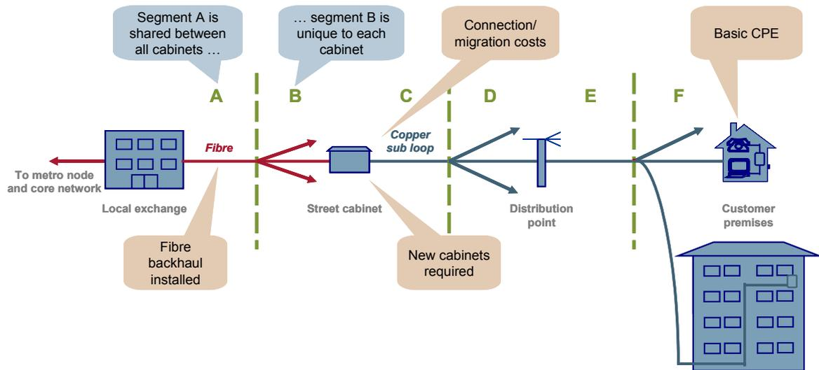
Figure 3.1: FTTC/VDSL network topology [Source: Analysys Mason for BSG]
