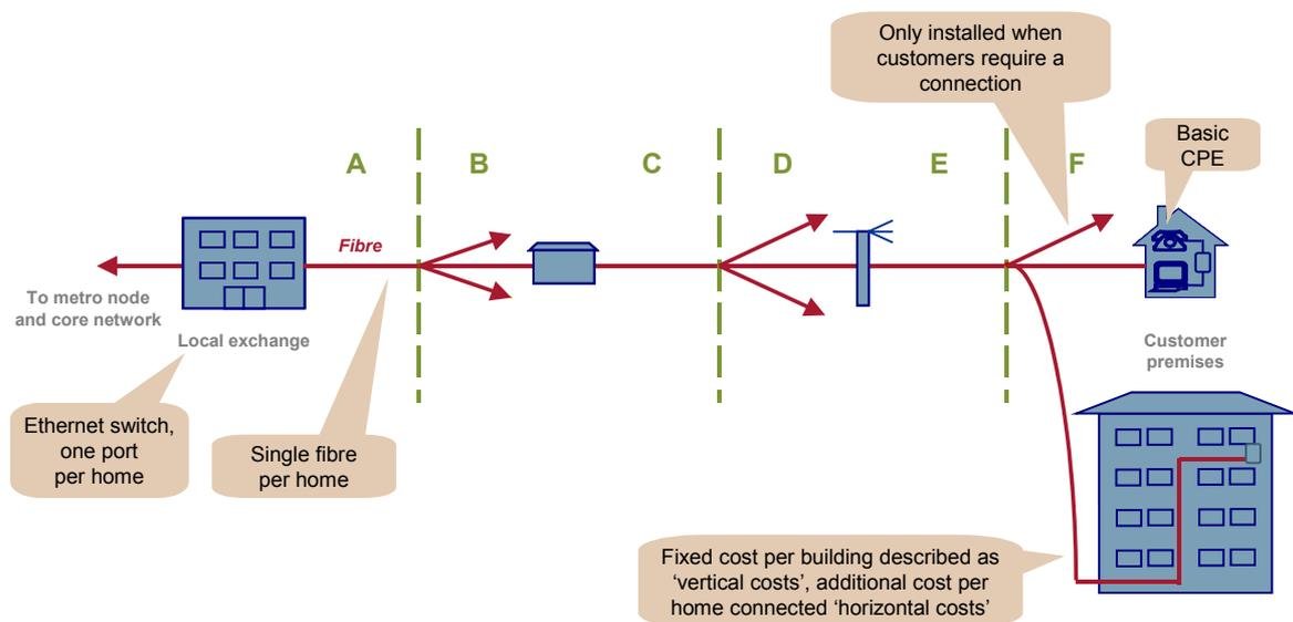
Figure 3.6: FTTH/PTP network topology [Source: Analysys Mason for BSG]
