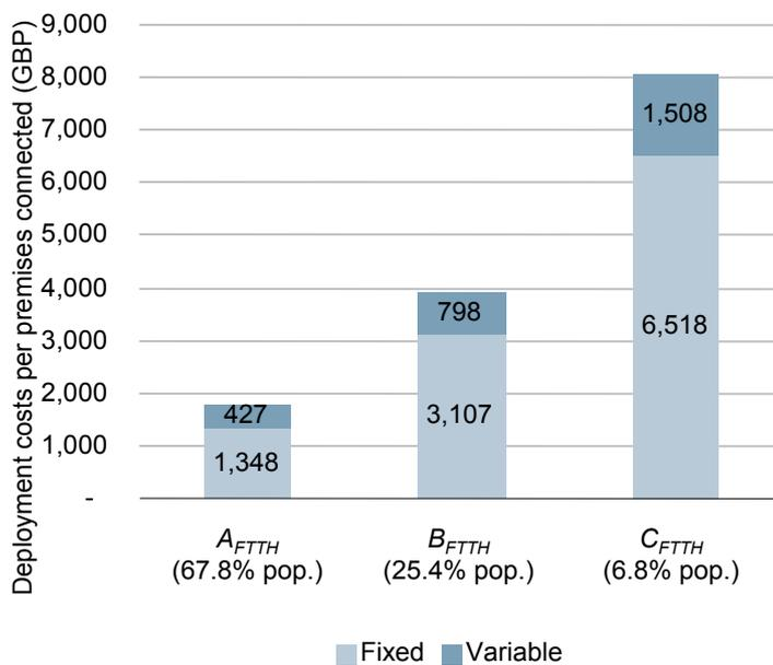
Figure 5.2: Fixed and variable costs per premises connected for FTTH/GPON split by geographical area [Source: Analysys Mason for BSG]
