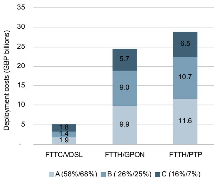
Figure 6.1: Deployment costs of each technology split by area (the corresponding population coverage for FTTC/FTTH is shown in parentheses)
