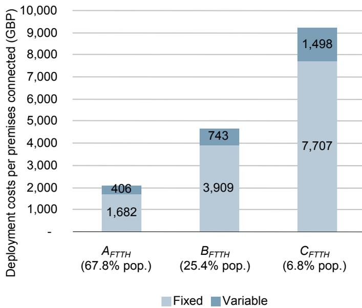
Figure 5.3: Fixed and variable costs per premises connected for FTTH/PTP split by geographical area [Source: Analysys Mason for BSG]
