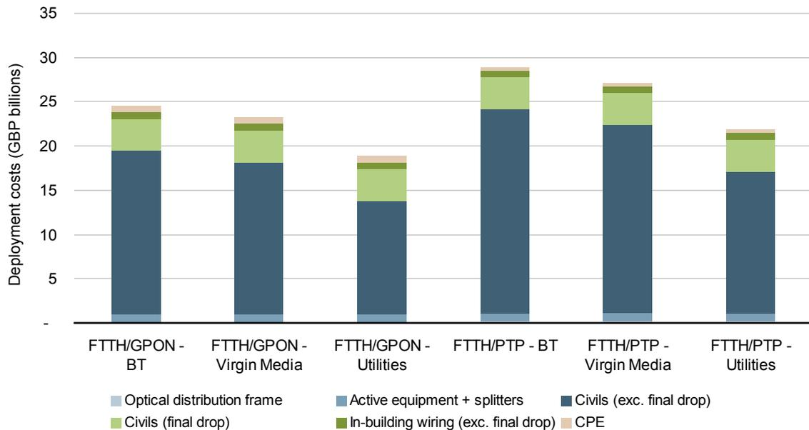
Figure 4.26: Deployment costs for a national network the different infrastructure scenarios for FTTH/GPON and FTTH/PTP [Source: Analysys Mason for BSG]
