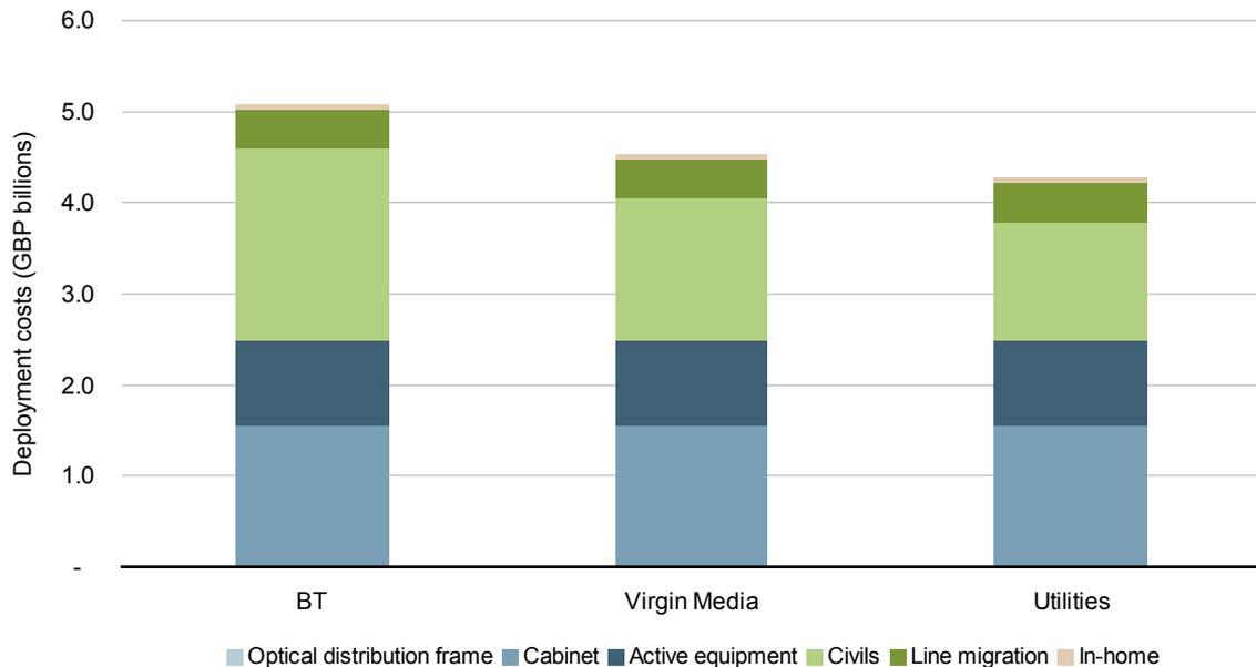
Figure 4.25: Comparison of deployment costs on a national basis for the different infrastructure scenarios for FTTC/VDSL [Source: Analysys Mason for BSG]
