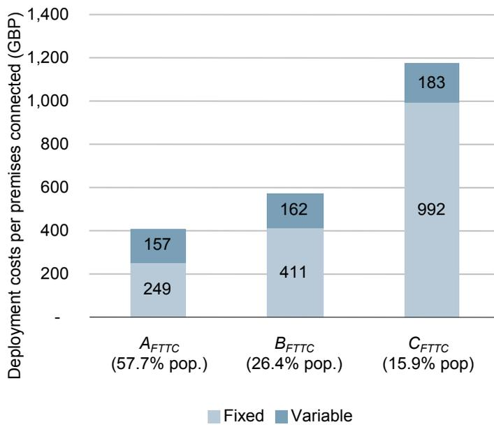
Figure 5.1: Fixed and variable costs per premises connected for FTTC/VDSL split by geographical area [Source: Analysys Mason for BSG]
