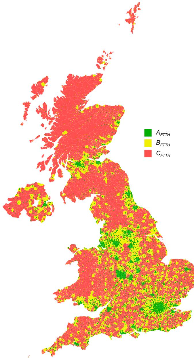
Figure 5.5: Map of the UK by area type for FTTH/GPON and FTTH/PTP [Source: Analysys Mason for BSG]
