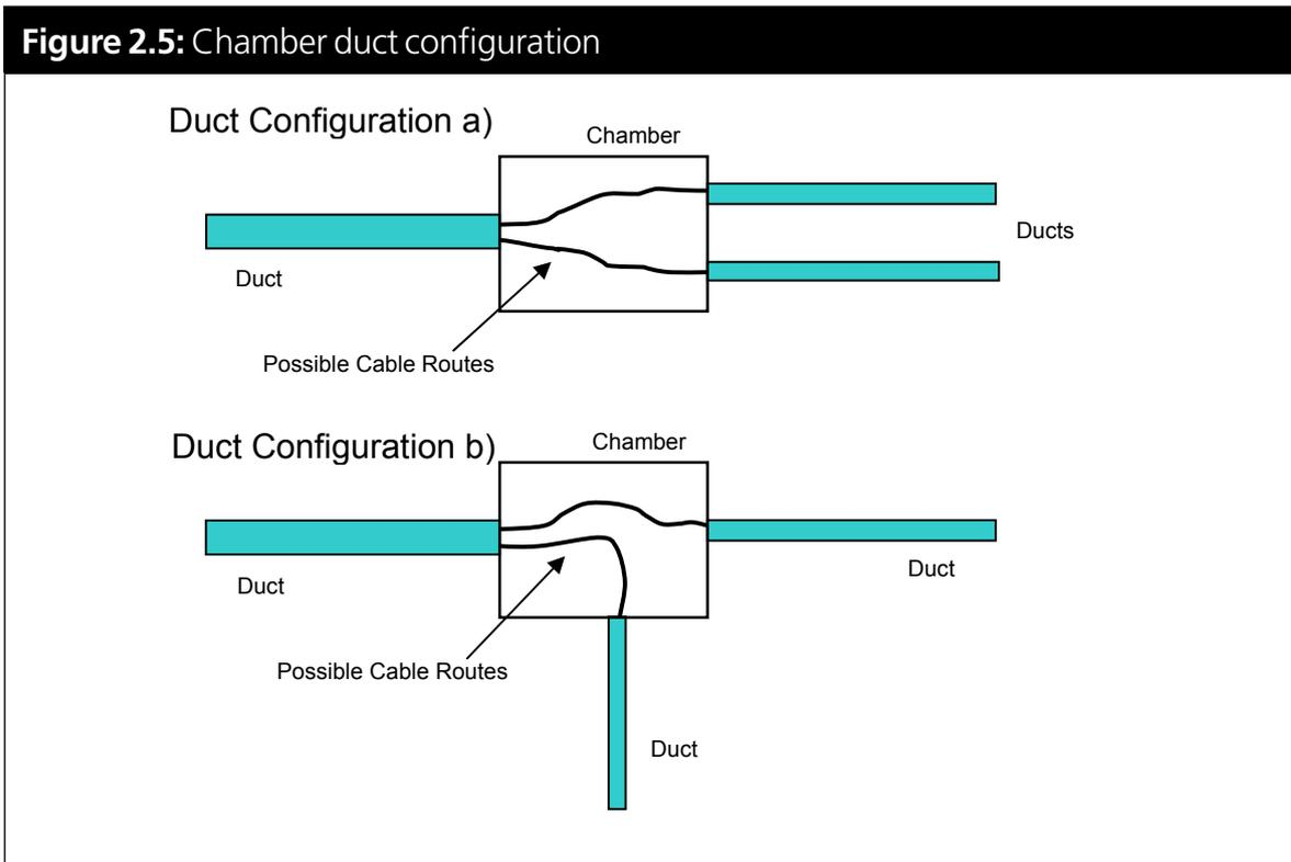
Developers should also consider the use of smaller chambers that can be used to pull cables on long duct runs (but under the maximum chamber spacing advised above).
