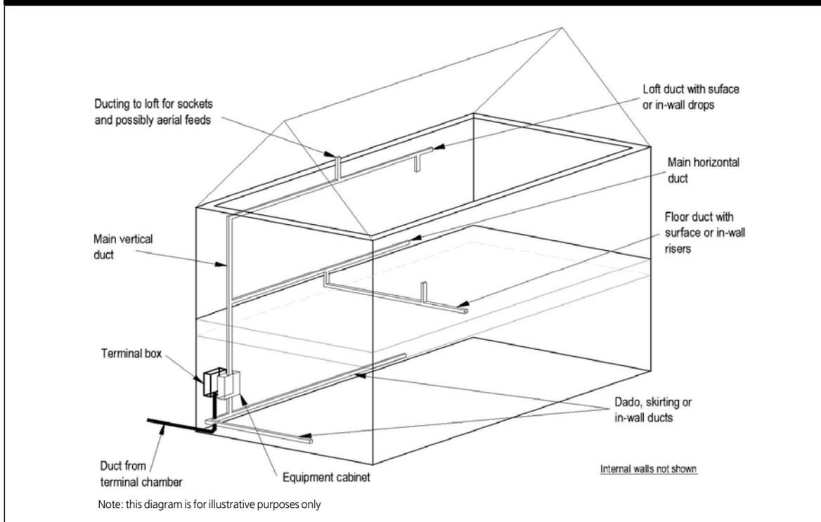
The ducts should be installed such that later cabling, and associated faceplates and sockets, can be installed with minimal disturbance to either previously installed cables or the fabric of the building. The aim should be to facilitate cable installation by an electrician or a qualified competent person.
